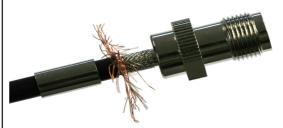
**6.** Insert the so prepared cable end into the connector housing as far it goes (click).
