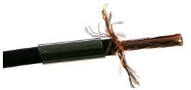
**2.** Remove 16mm of the outer sheathing with a knife. Bend copper braid upwards right-angled.
