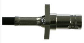
**8.** Crimp the crimp sleeve with a crimp tool; herewith the copper braid will be clamped between the socket housing and the crimp sleeve.
