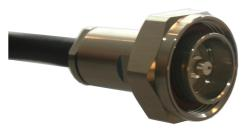
Push the prepared end of the cable into the connector housing as far as it will go. Hand-tighten the clamping nut with two open-end wrenches 17 mm and 18 mm. A small gap between the nut and the connector housing should still be visible! Then screw the contact onto the center conductor.
