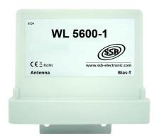
The WL5600-1 is a bidirectional amplifier for the WLAN frequency range 5.18GHz to 5.825GHz. It is equipped with an automatic transmission / reception switch. The gain is min. 25dB. A gain of at least 15 dB is ensured in the receiving direction. The output power can be up to 30dBm (1W).
