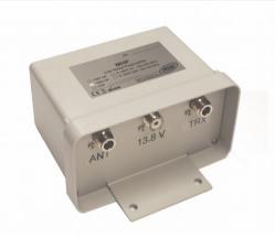
The **MHP 200** is a low-noise, large-signal-proof mast preamplifier with transmit / receive switching. It is intended for use in transmitting and receiving stations of medium and high power.
