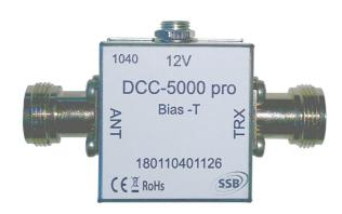
The DCC-5000pro DC switch is required to power amplifiers via the coaxial cable (remote feed). The HF-compliant design of the switch assures a high isolation between the HF-part and the DC-connection of the switch. The use of a low-loss microwave substrate and high-quality components guarantees low transmission loss and good adaption in the frequency range from 10 MHz to 6 GHz.
