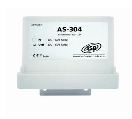
The antenna switch AS-304 is an electrically operated switch for four antennas. The unit is built into a weaherproof housing with mast mount. The switch is equipped with highly loadable power relays. In the result this High Frequency Switch is recommendale for a variety of tasks due to its big frequency range and the high power capacity. The according antenna is selected by simply putting the operating voltage of 12 V DC to one of the three Plus-PINs of the DINconnector.
